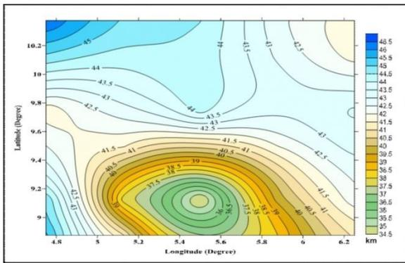
Fig. 11: Final Crustal Thickness Contour Map of the Study Area. [Contour Interval Is 0.5 Km. Colour Bar at the Right Indicate Values of the Crustal Thickness in the Area] where  $H_c$  is the crustal thickness in kilometres and BG is the Bouguer anomaly values in mGal
