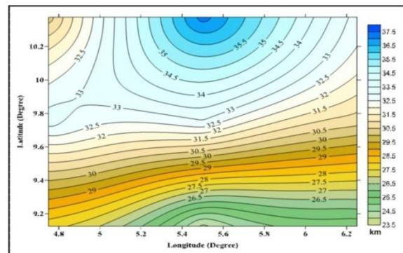
**Fig. 10: Contour Map of the Depth of the Conrad (H<sub>2</sub>) from Spectral Method over the Study Area. [Contour Interval is 0.5 km. Colour Bar at the Right Indicate Values of the Crustal Thickness in the Area]**
