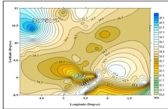
**Fig. 6: Woolard and Strange (H<sub>ws</sub>) Contour Map of Crustal Thickness of the Study Area. [Contour Interval is 0.2 km. Colour Bar at the Right Indicate Values of the Crustal Thickness in the Area]**
