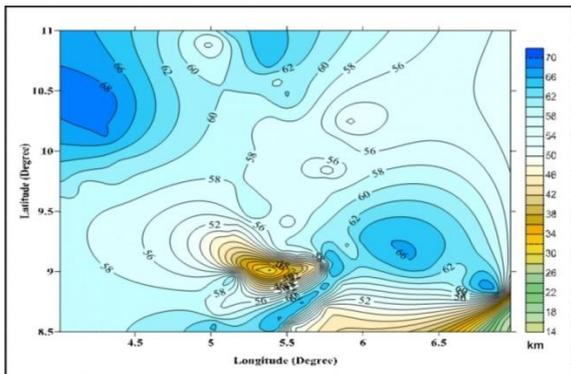
**Fig. 4: Demenistskaya (H<sub>D</sub>) Contour Map of Crustal Thickness of the Study Area. [Contour Interval is 2 km. Colour Bar at the Right Indicate Values of the Crustal Thickness in the Area]**
