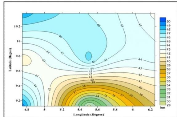
**Fig. 9: Contour Map of the Depth of the Moho (H<sub>3</sub>) from Spectral Method over the Study Area. [Contour Interval is 1 km. Colour Bar at the Right Indicate Values of the Crustal Thickness in the Area]**
